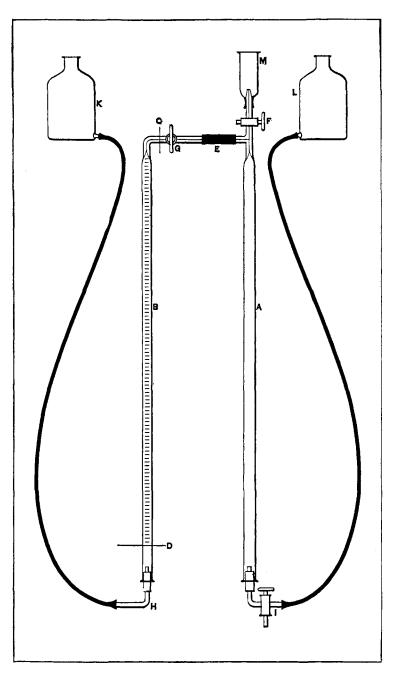
zero point, and the stop-cock G is closed. The excess of gas in A is expelled by opening the stop-cock F and raising the bottle L. The gas remaining in the capillary tube between C and the vertical part is disregarded, or its value may be ascertained and an allowance made; but usually it is too trifling to be worth notice.
